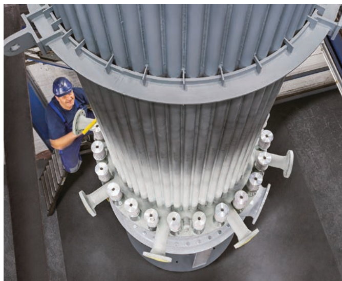
↑ Membrane wall of a HCl synthesis unit (S-1200e) with steam generation
