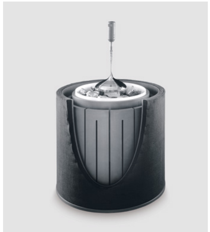
↑ Setup of a CZ crystal growth application with SIGRABOND Filwound susceptor, SIGRAFINE heater and SIGRATHERM GFA soft felt insulation
